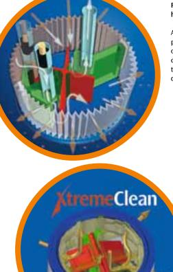
Powerful air pulses clean the filter gently and keeps suction performance constantly high – XtremeClean filter cleaning technology.
