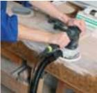
Our safety vacuum systems have been tested in accordance with the appropriate standards for ATEX Zone 22 or Zone 2. ONLY TYPE 22 accessories must be used to ensure continued conformity to the standards.
