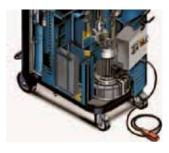
The side-channel suction unit is made of aluminum casting and fitted at the base of the chassis, giving more stability to the machine. The impeller is directly driven, thus avoiding any transmission and maintenance.
