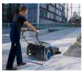
FLOORTEC 350 B is a battery-powered walk-behind sweeper with dust control and traction. Main and side brooms, filter, battery and on-board charger ready for use as standard. Suitable for service stations, car parks, playgrounds, factories, small warehouses, office buildings, hotels and conference halls.
