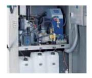
The AUTO BOOSTER is equipped as standard with an internal heater and cabinet insulation for protection against cold weather. Frost protection ensures the same level of protection in even lower temperatures.
