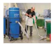
ATTIX 145 & 155 features a powerful double stage side-channel blower for heavy industrial vacuum cleaning in mechanical, ceramics, food and chemical industries. The all-steel construction secures a strong and reliable machine with high mobility, big capacity and storage facilities.
