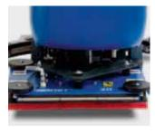
With SCRUBTEC BOOST, cleaning solution is introduced in front of the rectangular scrubbing pad/ brush and provides consistent contact via patented pulse solution control across the cleaning path. Using less water during cleaning keeps the operator working productively, rather than emptying and refilling the scrubber tanks.
