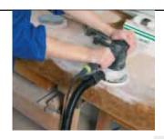
Our safety vacuum systems have been tested in accordance with the appropriate standards for ATEX Zone 22 or Zone 2. ONLY Type 22 accessories must be used to ensure continued conformity to the standards.
