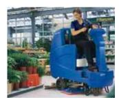
SCRUBTEC R 571 S, R 586 S and R 571 CS ride-on scrubber dryers are not only fun to operate, they are also the ideal solution for high speed scrubbing. They can be configured with different brushes, pads and other options to suit exact customer requirements. There are three models with cleaning paths of 71 cm, 86 cm and 71 cm with two cylindrical brushes.
