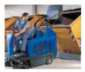
For easy emptying of the 130 L hopper, FLOORTEC R 680 is equipped with a hydraulic high-dump with a variable lift mechanism, to empty the hopper into containers of various heights. Max. lifting height is 1.8 m and emptying height is up to 1.5 m.
