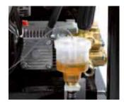
Easy oil drain from motor and pumps combined with low pump oil safety protects pump against running dry, keeping service costs low.
