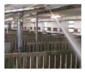
The easy to program MULTICLEANER 7-53 is an automatic washing robot with a built in high pressure washer. The MULTICLEANER is capable of doing 80% of the cleaning tasks in sheds. Sensors direct movement and optional kits allow the use of detergent and desinfection, or detect objects in the washing area. The robot is easily transported from one facility to another.
