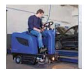
FLOORTEC R 670 is a robust sweeper designed to withstand tough working conditions – indoors or out. Excellent turning radius - for optimum work flow and up to 20% ramp climbing capacity.
