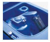
Easy-fill tank system allows the machine to be filled from nearest available water supply. The large cover and recovery tank opening make it very easy to clean.
