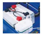
Optional chemical mixing system automatically mixes chemical stored in an on-board container with clean water stored in the machine's solution tank, and delivers the mixed solution to the brush deck for scrubbing application. The advantages are reduced costs and
