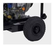
The large pneumatic wheels ensure good manoeuvrability over the uneven ground found largely on building sites and in agricultural environments.
