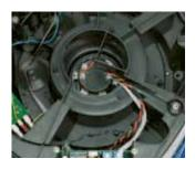
The EC drive system is a brushless longlife motor with electronic regulation and precise power control. A durable and efficient solution for continuous use without sparks or carbon dust from the motor.
