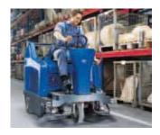
The FLOORTEC R 680 is a high capacity dust-free sweeper with a working width of 1050 mm, a powerful vacuum system and a 130 litre hopper for sweeping large floor areas without emptying. The FLOORTEC R 680 excels not only in productivity but also in climbing power. Ramp climbing up to 20% incline.
