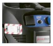
The built-in FlowSensor and acoustic warning signal monitor air speed in the suction hose to make sure that it does not fall below the minimum of 20 m/s. The use of suction hoses with different diameters is easily adjustable on the main control board.
