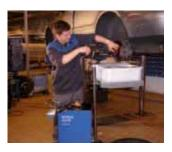
Cleaning takes place with the help of hot water and detergent under low pressure. In this way harmful dust, oil, grease and dirt are bound and removed in one operation. The B23 Stainless can be moved freely in the workshop – independently of water and power supplies. One filling of compressed air and detergent is sufficient for 10-20 cleaning jobs. The tray can be turned horizontally and the height adjusted. This means that the brake washer is suitable for lorries as well as cars.
