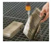
Washable PET filters and automatic/semiautomatic filter cleaning systems secure low downtime, continuously high suction performance and low maintenance cost – a machine build for professional use.
