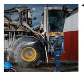
The POSEIDON 7 FA industrial class cold water high pressure washer combines the renowned lifetime and quality of the C3 pump with optimal ergonomics to bring an unbeatable heavy duty pressure washer for industry, agriculture, shipping, transport sector and food industry.
