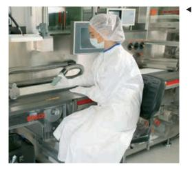
The ATTIX 50 CLEAN ROOM model is designed for use in clean room applications as found in hospitals, electronic laboratories and the pharmaceutical industry. A HEPA main filter and the additional motor cooling air filter provide high filtration of both exhaust working air and cooling air flows.
