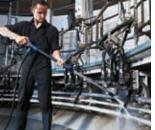
Nilfisk-ALTO stationary solutions are incredibly flexible. Through careful planning of the installation, it is possible not only to work in the general vicinity of the pressure washer, but also to work at various locations throughout your premises by using a pipework system, allowing one or more users to clean at long distances away from the machine.
