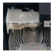
Pump oil sight and oil tank with integrated low pump oil safety cut out. Maintenance is simplified and the machine is protected against running the pump without oil, ensuring longer service life.
