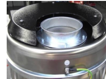
Exhaust air vent on top
