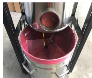
Dirt container with separator star
