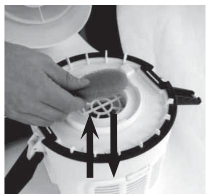
**Exhaust filter to be replaced
